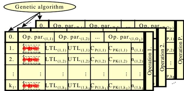
Fig. 4. The parameter set of the process optimization. For the  $j^{\text{th}}$  operation there are  $k_j$  “internal” parameters and  $O_j$  operation parameters
