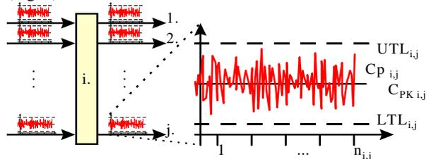
Fig. 2. Control charts adjusted to all of the input and output parameters of the operations
